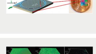
Laser-induced graphene (LIG) has been shown to be effective in resisting biofouling (the buildup of biological material on wet surfaces) and, when used as electrodes
