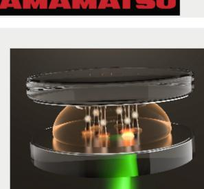
bounced back and forth rapidly between two mirrors. Researchers placed a dyepolymer solution within an ultrahigh-finesse microcavity between the mirrors,
