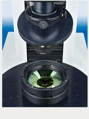
analysis of bubbles and inclusions for optical substrates in the Visible and NIR wave-bands (works for most IR glasses). This instrument enables full quality assurance and reports to
