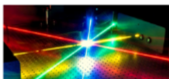
OPO technology provides laser light that is widely tunable across the visible spectral range. Figure courtesy of Jens Essling (Physikalisches Institut für Physikalische Messtechnik).
