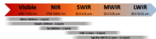
Figure 1: The various sub-regions of the electromagnetic spectrum, covering visible through to infrared wavelengths. Some common detector materials and their typical wavelength detection ranges are also listed.
