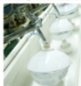
Figure 1: Full aperture polishing of spherical surfaces
