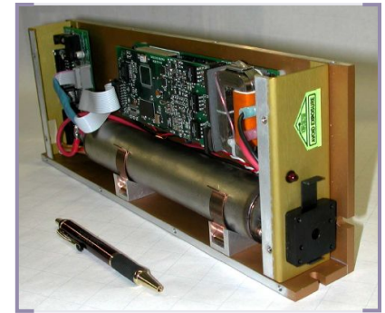
Series 30 Laser with integrated controller (cover removed)
