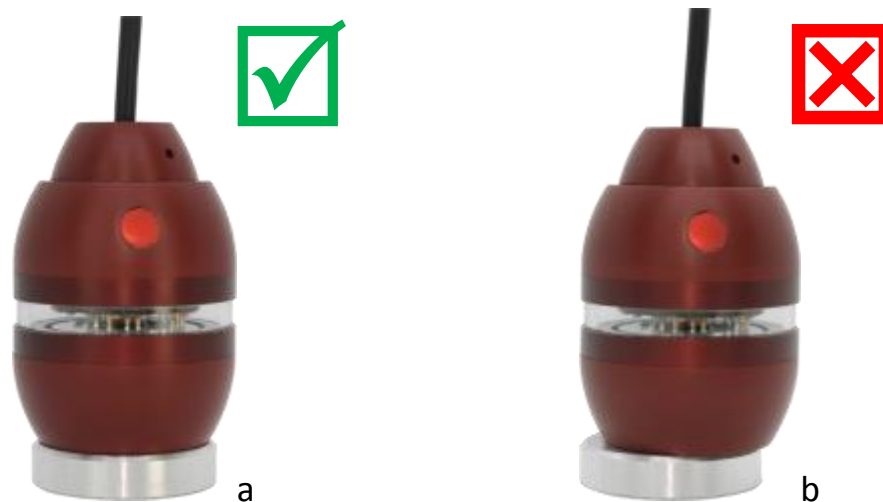
Fig. 4. Minispectrometer orientation relative to the etalon at calibration measurement: a – correct, b - incorrect.
