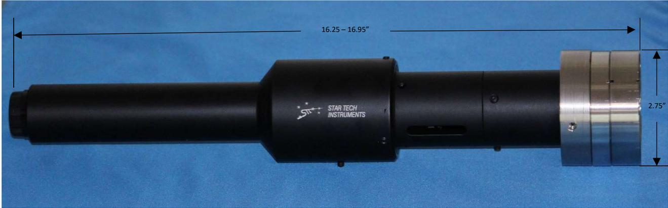
The μBIP series is STI's latest imaging system designed specifically for use with soft x-rays [1-2 nm]; it cannot be used for longer wavelengths such as 193 nm or 248 nm from excimer lasers which would cause severe internal damage. Most importantly, the system is designed for use with high vacuum chambers using our custom vacuum flange assembly for attaching the optical system to the vacuum chamber. The flanges are rated at  $\geq 10^{-8}$  Torr.
