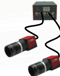
Streamer with no internal camera, 2 x U750 cameras connected via single cables to Streamer Controller.
