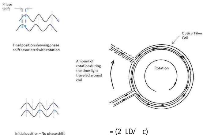
Initial position – No phase shift associated with counter propagating waves
