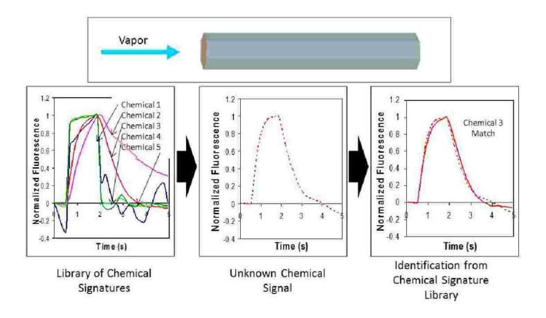
Figure 16.14 Fluorescent Array Microsphere Vapor Sensors<sup>10</sup>
