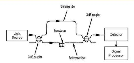
Mach-Zehnder interferometer configuration
