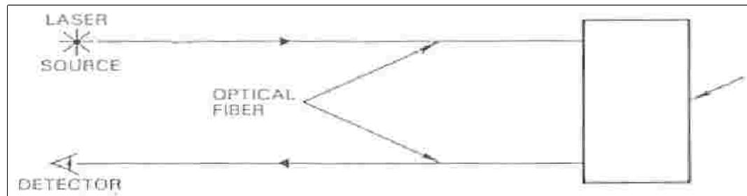
Fiber carries light in and out of the device
