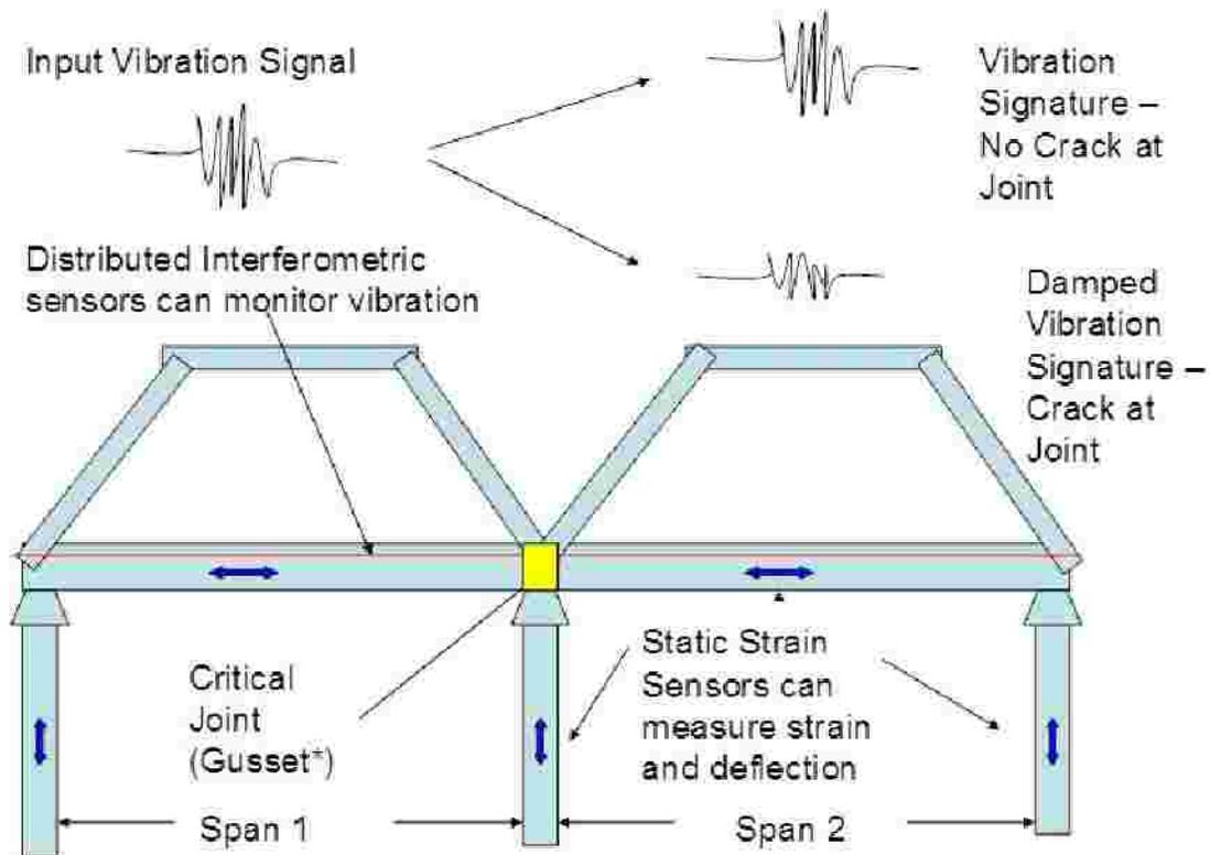
\* Suspected failure point in Minneapolis bridge failure
