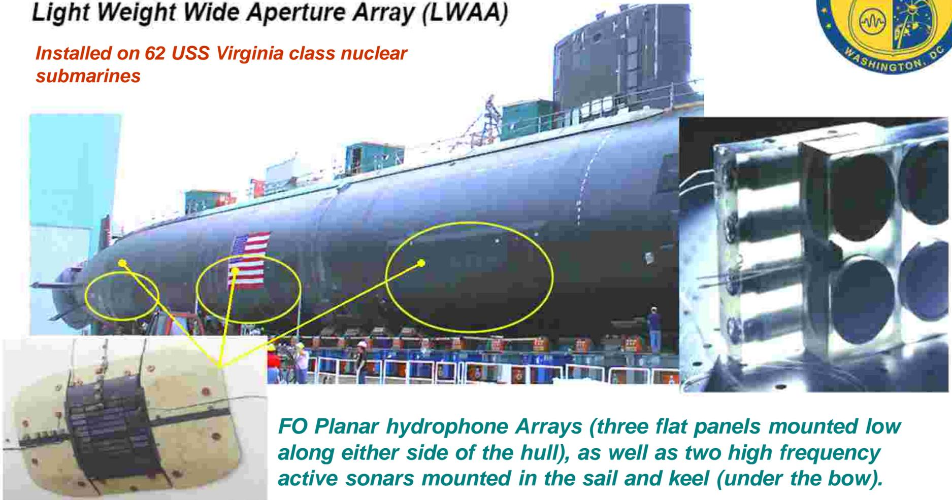
**FO Planar hydrophone Arrays (three flat panels mounted low along either side of the hull), as well as two high frequency active sonars mounted in the sail and keel (under the bow).**
