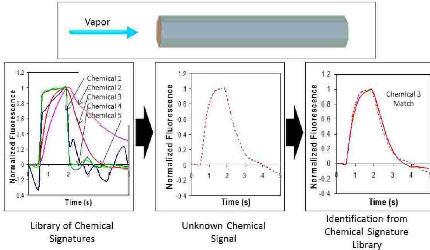
Figure 16.14 Fluorescent Array Microsphere Vapor Sensors<sup>10</sup>
