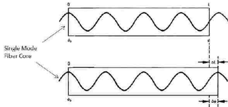
Phase change of a light wave through an optical fiber of original length  $L$  that has been stretched by a length  $\Delta L$
