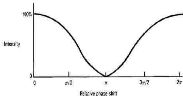
Intensity versus relative phase shifts due to constructive and destructive interference
