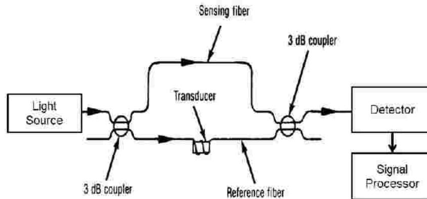
**Mach-Zehnder interferometer configuration**
